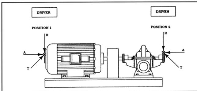
Figure 1 - An external schematic showing the transducer locations.
